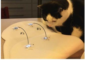
5) Flip UnderFlap area of Foam UP toward OverFlap area. Place one "A" & one "B" magnet piece within the circled areas indicated with their magnetized and marked side facing UP. Please note that in this arrangement, the "A" pairs should be matched on the left side of the Foam (and the "B"s on the right). Double check to make sure this is the case, (or ask your assistant to check for you), then stitch them in place and set your Foam aside for step 33.
